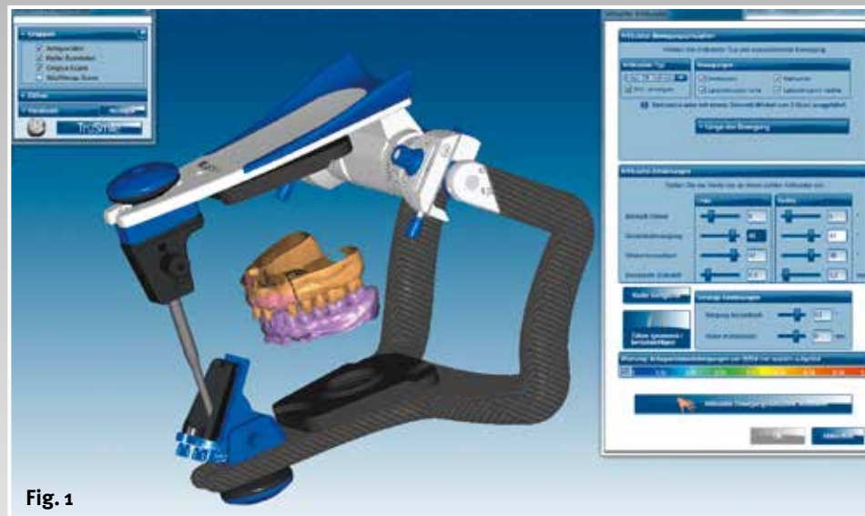
► Fig. 1 Starting point of all design elements: the Artex CR virtual articulator
