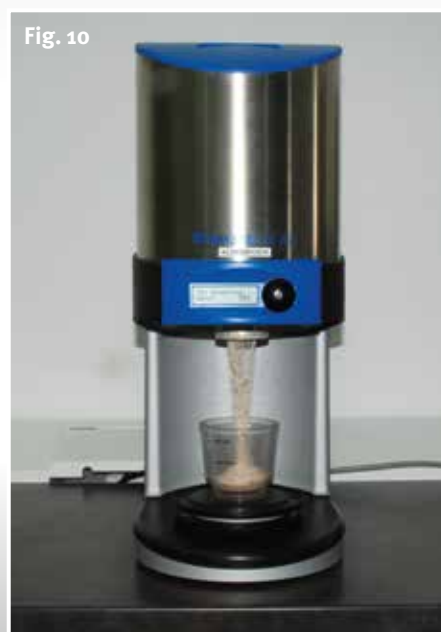
▶ Fig. 10 Smartmix X2 from Amann Girschbach; an automatic mixer for accurate dispensing of water and plaster to ensure exact control of the plaster expansion
