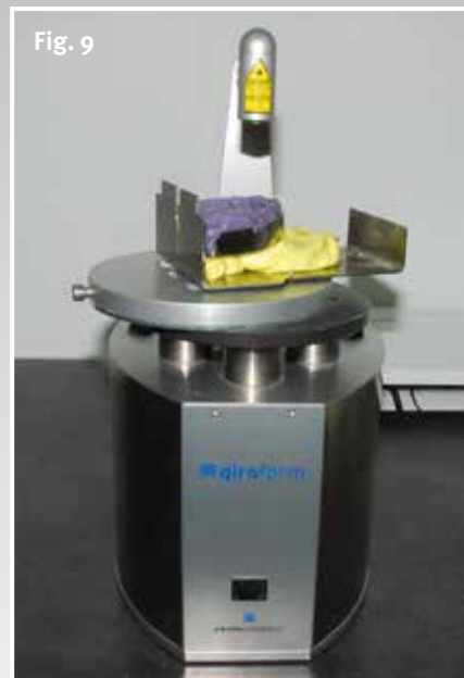
▶ Fig. 9 Giroform model fabrication from Amann Girschbach, based on the Giroform pin-drilling unit and plastic baseplates for the sectioned model
